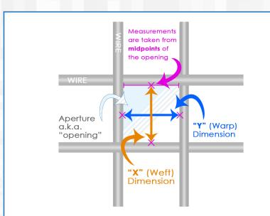
Each sieve is scanned by sophisticated optical technology and software which takes accurate aperture (opening) measurements in the "X" and "Y" directions (warp and weft). Wire diameters are also measured to ensure compliance with ASTM E11 specifications.
